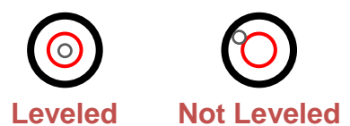
Figure 5-2-3. Leveling Spirit Level
