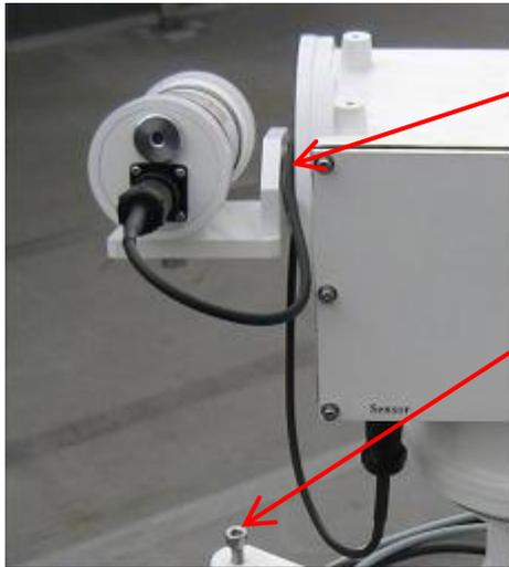
First place the signal cable on the Driving Part axis then connect the cable ends to each connectors.
