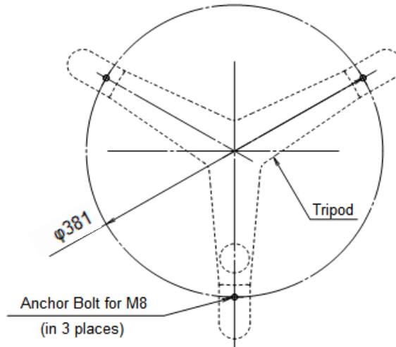
Figure 5-3. Anchor bolt position
