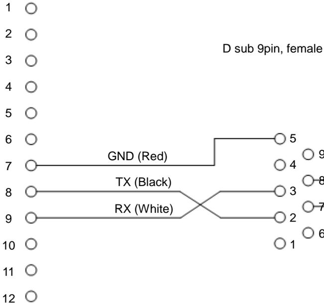
Figure 8-1. Communication cable & Pin Assignment
