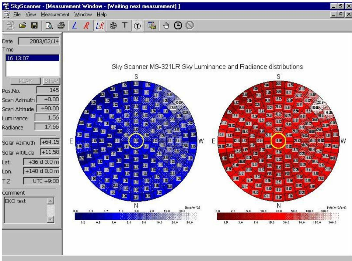
Figure 6-8. Example of Display during Measurement
