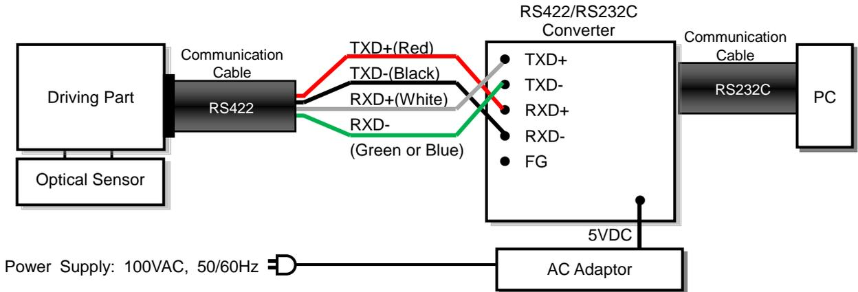
Figure 5-6. RS422/RS232C Converter Connection for Using Extension Cable
