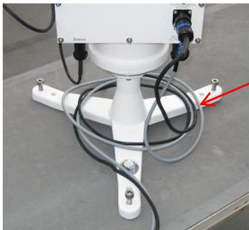
Run the power cable and communication cable twice around the tripod with sufficient length as shown on the left.
