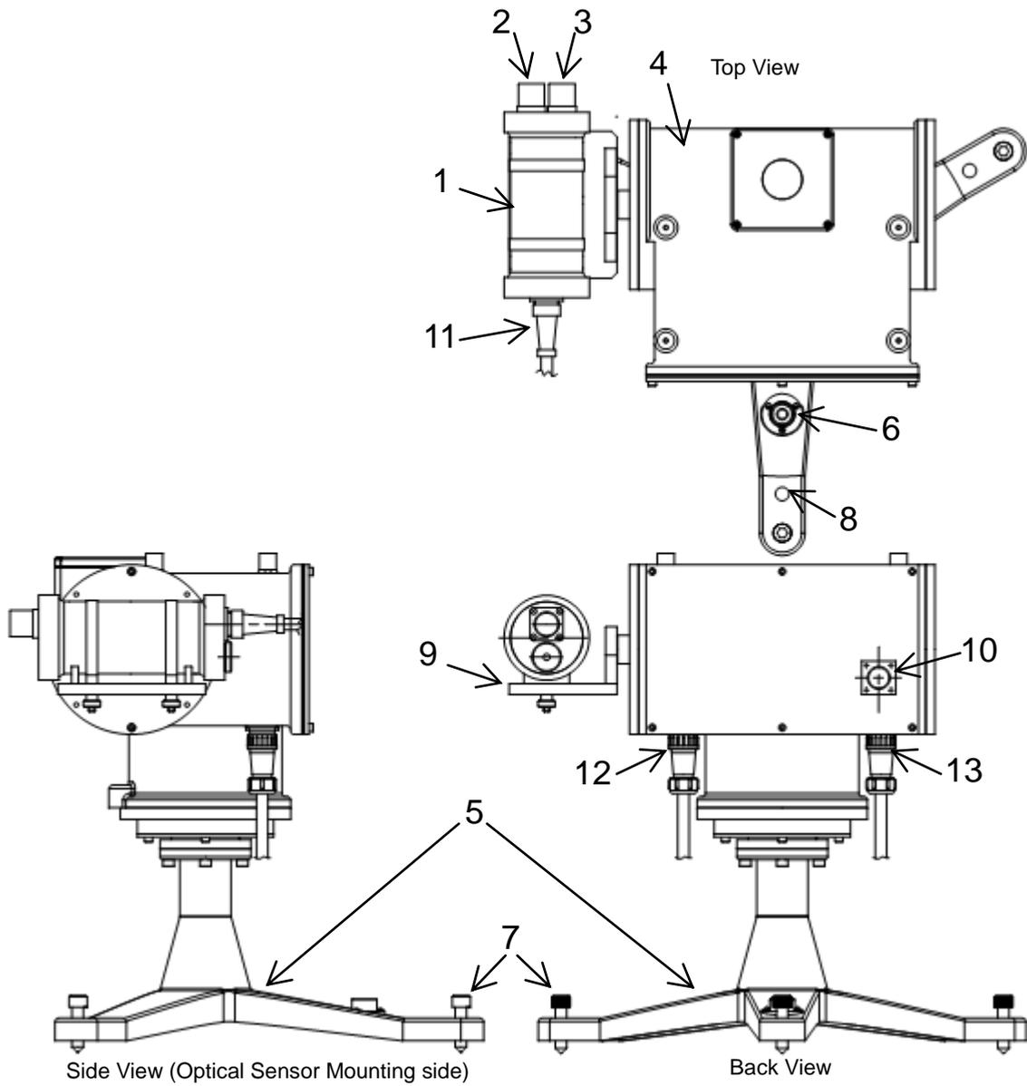
Figure 5-1. Sky Scanner Parts Name and Functions
