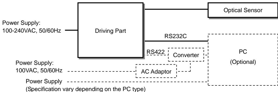
Figure 5-2. Sky Scanner Block Diagram
