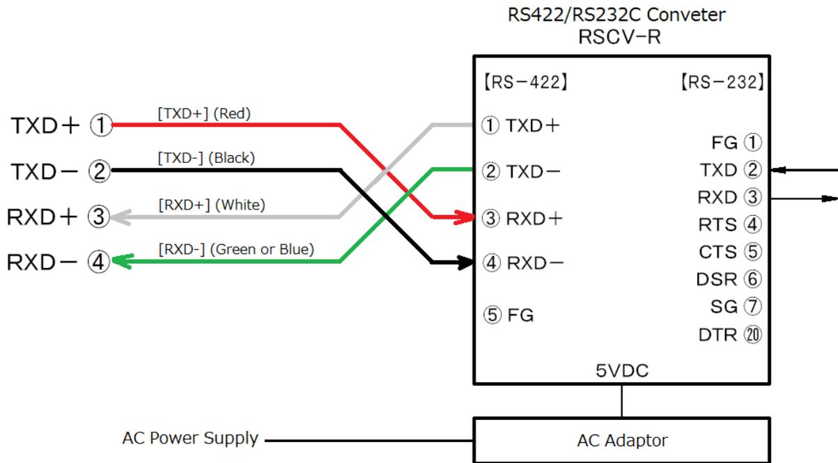
Figure 5-7. Signal Flow Diagram
